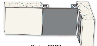
Series FSWL Corner Wall / Concealed Mud Frame Nominal Joint Openings 1" to 2"
