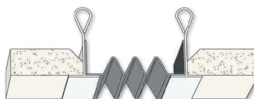
Series DX Ceiling-to-Ceiling Nominal Joint Openings 1" to 2"
